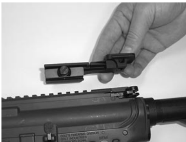
Figure 3-1 Attaching Weapon Mount to Weapon
